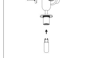
Insert a G9 light source into the socket. Make sure to press the light bulb all the way into the socket.
