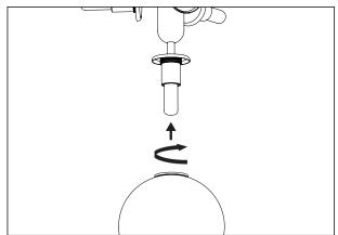
Carefully place the glass globe over the light bulb. Turn clockwise to attach the glass globe.
